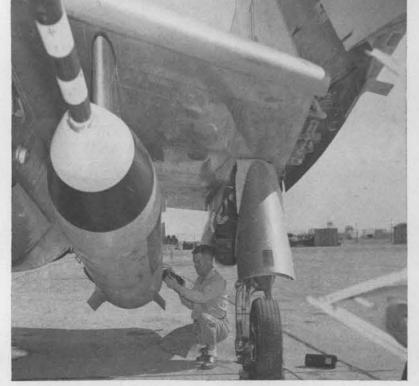
CAMERA INSTALLATION is the task of Dean Heath, who works here on an RP (research parachute) shape hanging on a Cutlass.
